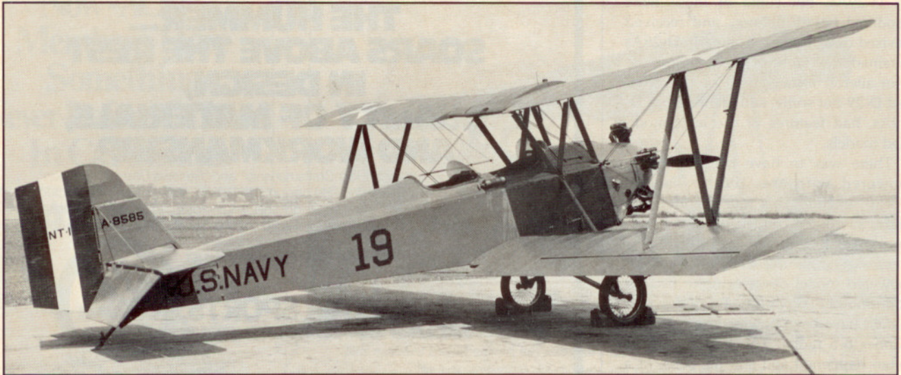
The Navy's six NT-1s (D-29As) were equipped with wire wheels and improvements such as two conventional cockpits and ailerons on the lower wings only (above). The sole surviving New Standard D-29A (below) retains the original bathtub cockpit and still is flying.
