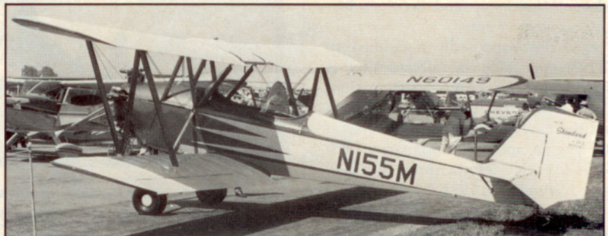
The Navy's six NT-1s (D-29As) were equipped with wire wheels and improvements such as two conventional cockpits and ailerons on the lower wings only (above). The sole surviving New Standard D-29A (below) retains the original bathtub cockpit and still is flying.
