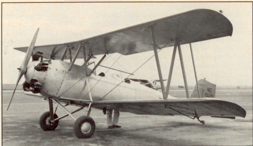
This modified D-29A (above) has a rounded fuselage, two cockpits, metal paneling from the nose to behind the cockpits and fairing strips from the rear cockpit to the tail. Another modification of the D-29A is shown below. Note the wind-driven generator above the landing gear used to power the lights.
